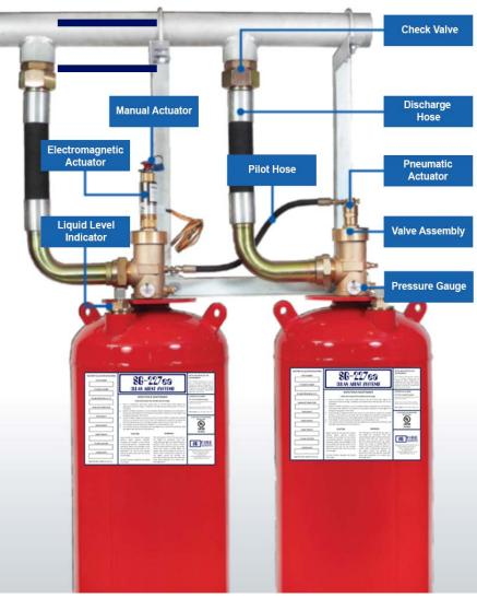
The SG-227ea cylinders are available with both Mild Steel Welded type of TPED 2010/35/EU Standard and Chromium Molybdenum Alloy Steel Seamless type of ISO 9809-1 Standard. SG-227ea is a product of SG Fire Systems from Singapore.
